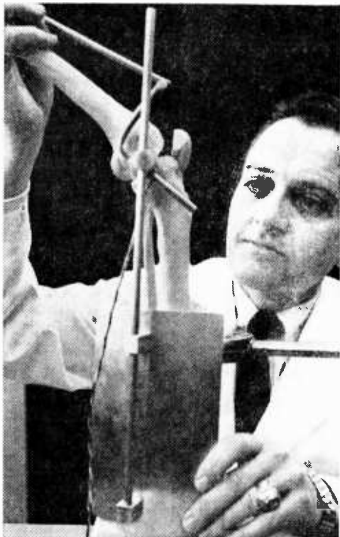
Device above records knee motion, passes findings on to computer for analysis. Knee in photo is model.
